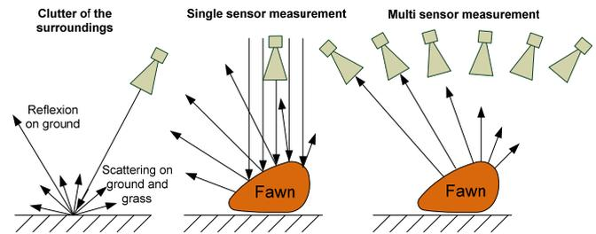
Fig. 3 Microwave signal scattering from the fawn and the ground
