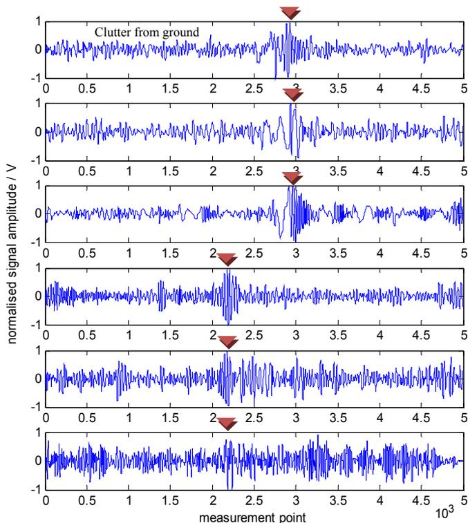
Fig. 6 Doppler signal measurement with six receiving antennas and one transmitting antenna (three transmitting antennas pointing in moving direction, the other three backwards,  $\blacktriangledown$ : target object, TX and RX antenna height = 80 cm, TX-RX antenna distances = 20 cm, 60 cm, 120 cm)
