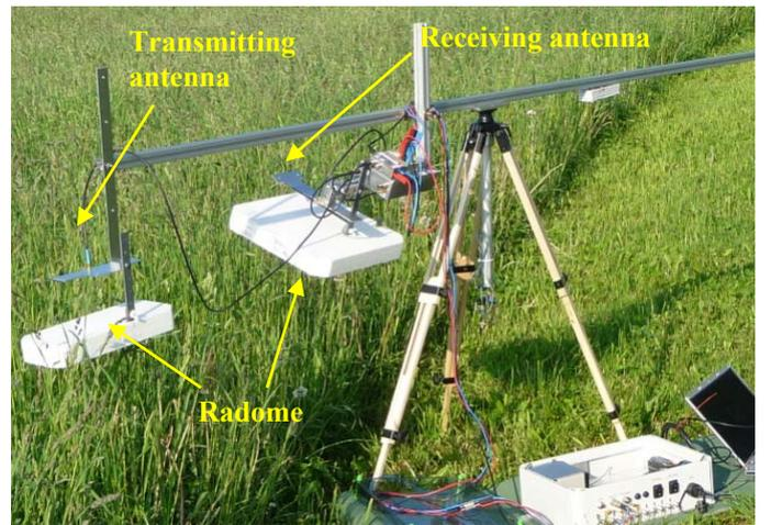
Fig. 5 Multistatic radar measurements with a tripod
