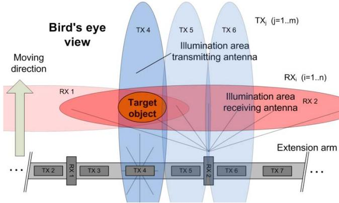
Fig. 4 Antenna arrangement of the multistatic radar
